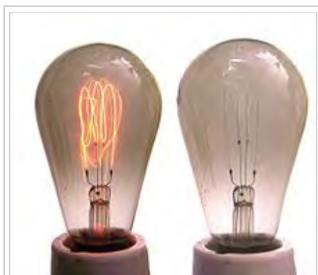
Carbon filament lamps, showing darkening of bulb
