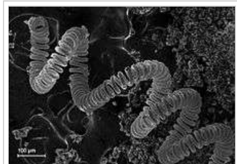
SEM image of a tungsten filament of incandescent light bulb.
