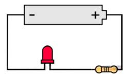
A good resistor value for most LEDs is 330 Ohms. You can use the information from the last section to help you determine the exact value you need, but this is LEDs *without* math... So, start by popping a 330 Ohm resistor into the above circuit and see what happens.
