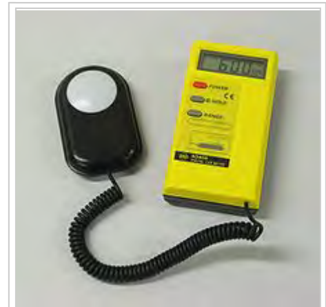
A lux meter for measuring illuminances in work places.
