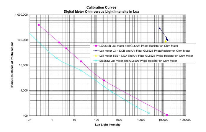
Photo resistor GL5506 works better for measuring low light intensities. For accuracy one needs to do ones own testing. For there is a wide range of different ohm values for the same model photo resistors, with each individual having a different calibration results.
