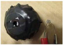
This UVC light sensor (shown on the right above) was made using (front to back) a fender washer with a ¼" hole in it, then the UV pass ban filter then the photo resistor. This was embedded in black foam rubber. Enough black tape was used on the outside to keep light from coming in form the side. Sun light being very high intensity parallel waves from one direction was used to test for leakage by slowing turning the sensor to different direction and watching the ohm meter.
