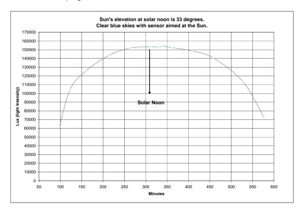
Maximum intensity at solar noon on a clear day after rain was measured to be about 126,000 Lux to 156,000 Lux depending on what meter was used. It is not known witch one is closer to a standard calibration. Be aware your meter may also be off in calibration and that it would be wise to take some of your own readings before the pole shift.
