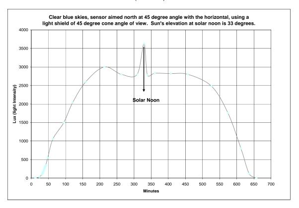
It is interesting to note there is a bounce effect that increases the light intensity at or near solar noon. This curve represents reflected light from a light blue sky. Note, it is still very much lower in intensity than the direct sun.
