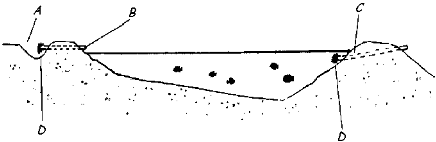
Figure 35: Cross-section of the water inlet and outlet of a pond (Murnyak and Murnyak, 1990). A: silt catchment basin; B: overflow pipe; C: inlet pipe; D: screen.
