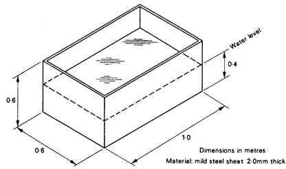
To find the mass of the open-topped container shown together with water filled to a depth of 0.4 m
