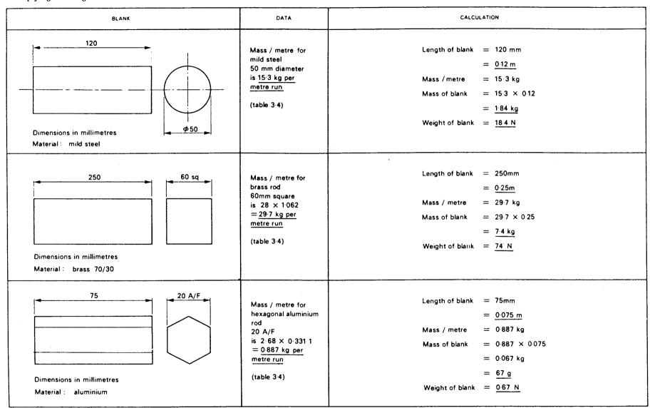
Fig. 3.6 Calculation of metal blank weights (bars)
