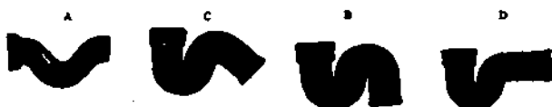
FIG. 220.—Different Forms of Traps. A, Running trap; B, S-trap; C, † S-trap; D, ‡ S-trap.
