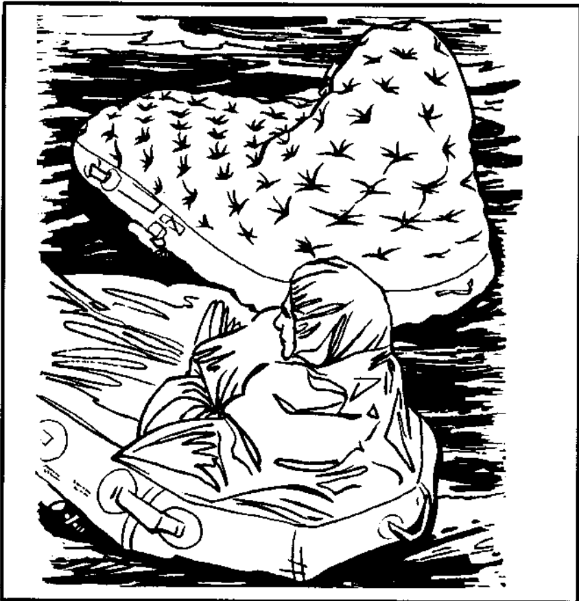
Figure 16-11. One-man raft with spray shield inflated.
