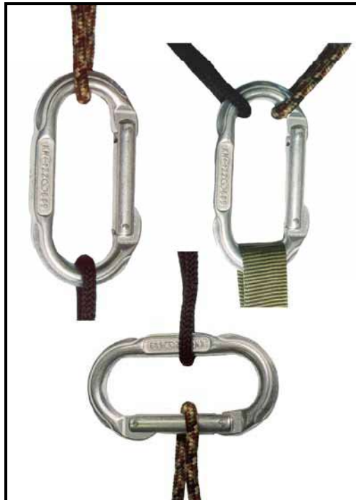
Figure 3-12. Major and minor axes and three-way loading.
