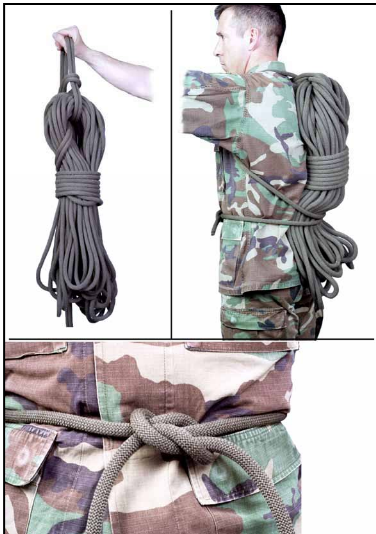
Figure 4-5. Butterfly coil tie-off.
