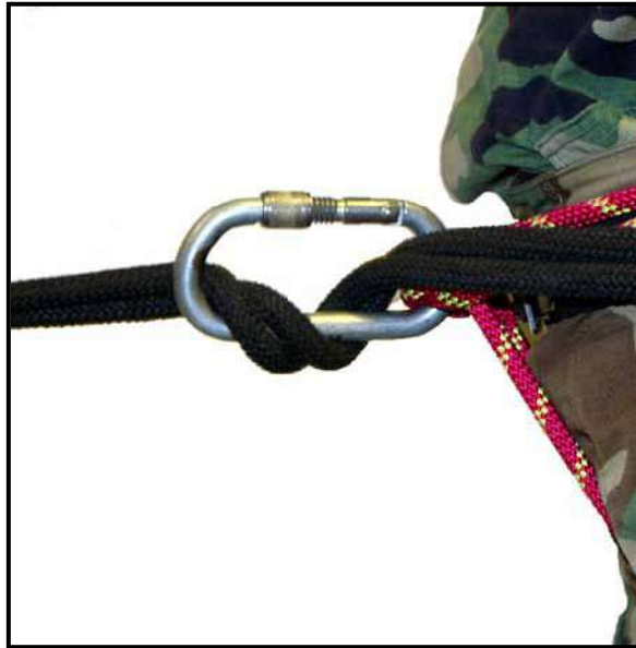
Figure 7-7. Proper hookup using carabiner wrap.
