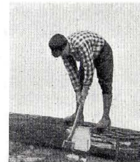
Fig. 21.—Second stroke should place the axe in the lower side of log as shown.
