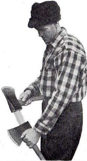
Fig. 17.—Drive in tightly a long wedge of well-seasoned wood. Then cut off the surplus wood and restore the Take-Up Wedges.
