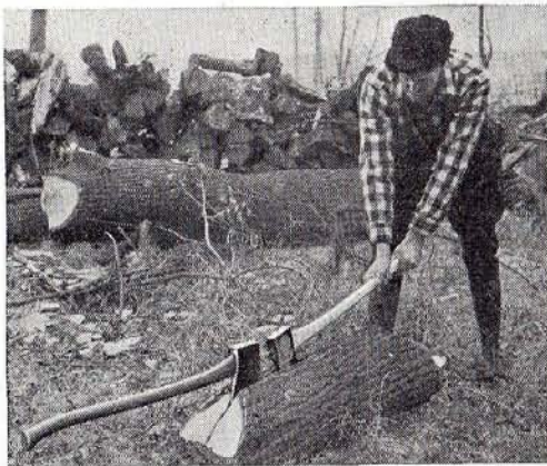
Fig. 25.—Splitting a log with two axes. One axe loosens the other as the chopper progresses up the log.
