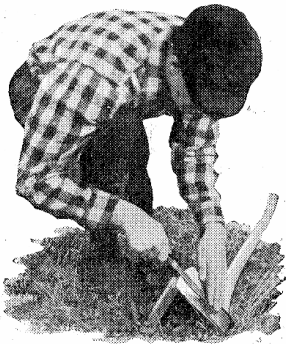
Fig. 7.—Hold the file level with the axe blade. Note the peg driven into the ground to hold the axe for sharpening.
