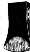
Fig. 5.— Fan grind, the best way. See the file marks running back towards the head.
