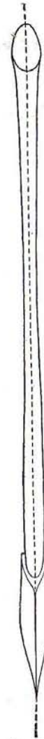
Fig. 16.—In a correctly hung axe, the cutting edge is in a direct line with the center of the handle.
