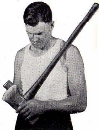
Fig. 10.—First position for honing the edge after sharpening.
