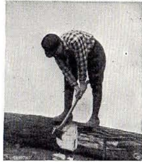
Fig. 22.—Third stroke places the axe in the middle of log and throws out the chip.
