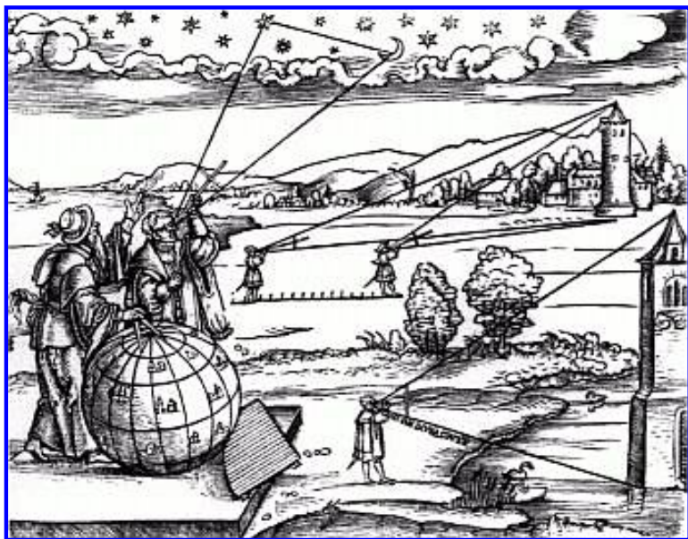
Cross-staff used for computing lunar distance and height of buildings
