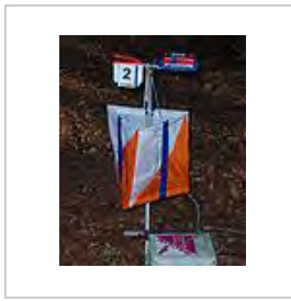
ARDF control point equipped with an electronic punch station and a radio transmitter that reports each use of the punch to a base station
