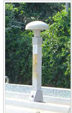
This antenna is mounted on the roof of a hut containing a scientific experiment needing precise timing.
