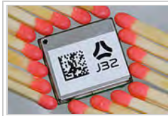
A typical OEM GPS receiver module measuring 15×17 mm.
