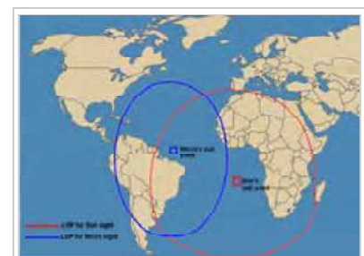
A celestial fix will be at the intersection of two or more circles.
