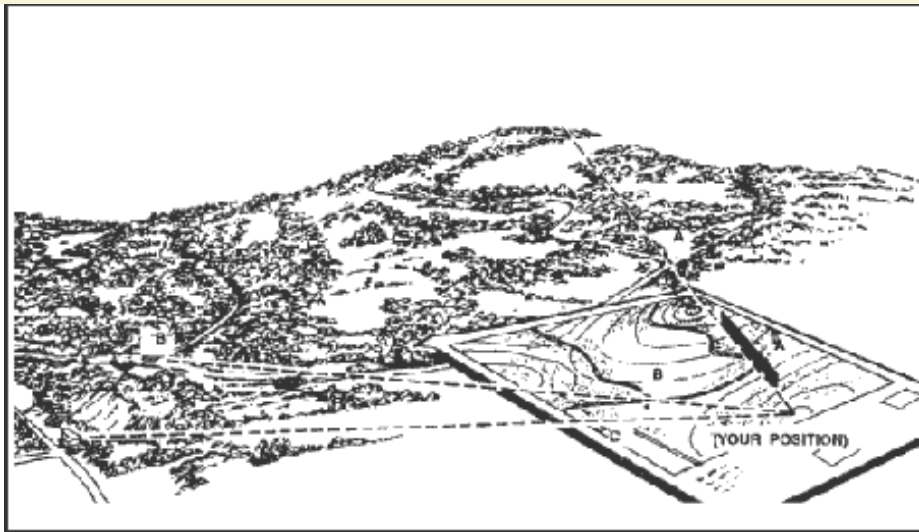
Figure 6-19. Resection with straightedge.
