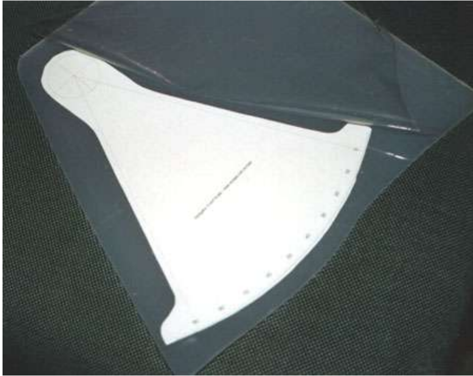
Lift the plastic protection, stick the scale, and put the protection back in place
