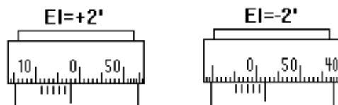
fig. 16 - Sign of the instrumental error
