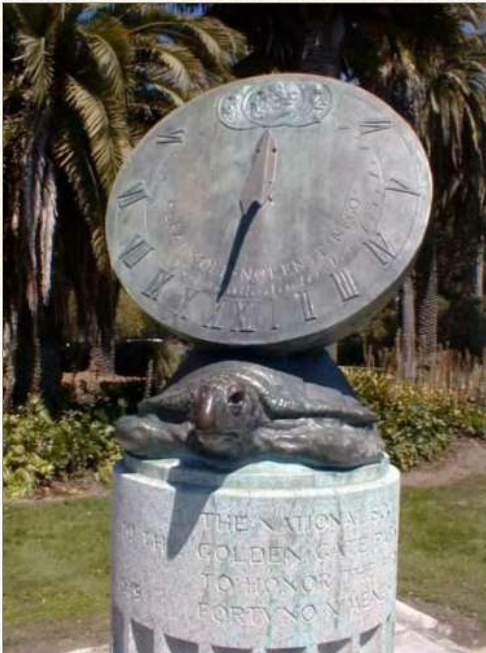
A reclining dial. The dial is oriented due south, but the face reclines from the vertical.
