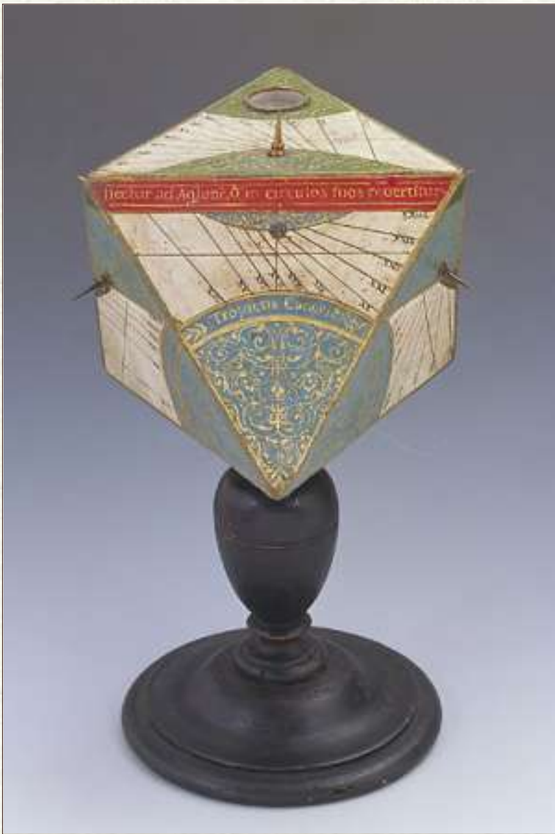
A polyhedral dial in the form of an octahedron. By Stefano Buonsignori, Florence, 16th century.
