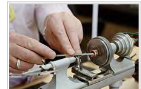
A watchmaker using a lathe to prepare a component cut from copper for a watch
