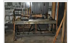
Water-powered Blanchard lathe used for duplicating gun stocks from 1850's. Harpers Ferry Armory.
