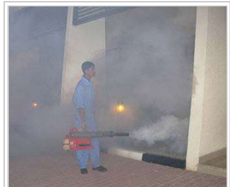
Space treatment against mosquitoes using a thermal fogger
