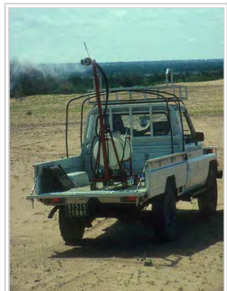
The Ulvamast Mk II: a ULV sprayer for locust control (photo taken in Niger)
