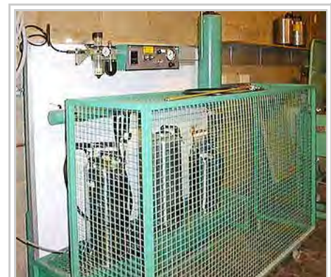
IPARC houses and carries out the World Health Organisation fatigue test for pressurised equipment: used for indoor residue spraying (IRS) against mosquitoes, other disease vectors and (sometimes) in agriculture
