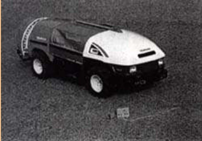
Fig.2. Unmanned sprayer, guiding cable, guiding signal generator and Palm-sized remote control transmitter
