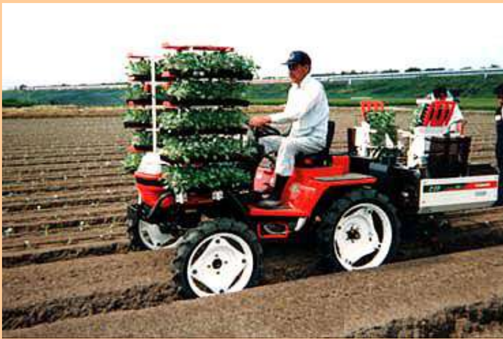
Fig.7. Fully automatic transplanter Model PR2 for cell mold seedlings (Yammer Noki, Co., Ltd, for cabbage in Ogoori, Fukuoka)
