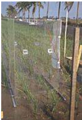
Photo 1: Closed chamber method for CH 4 flux measurements
