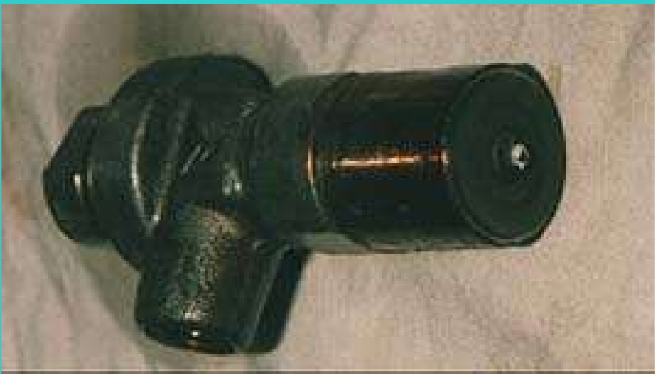
Fig.5. Injection nozzle after long-term operation using crude rapeseed oil
