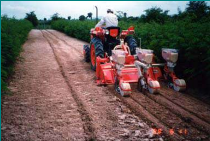
a): Seeding of corn with rotary drill seeder
