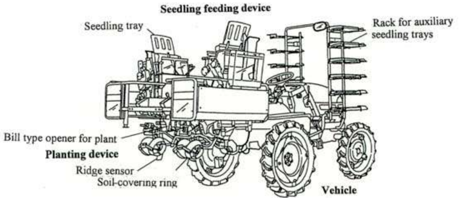
Fig. 2. Fully automatic transplanter model PR2 for cell mold seedlings
