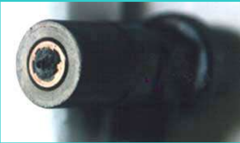
Fig.8. Injection nozzle after no-load continuous operation using degummed rapeseed oil
