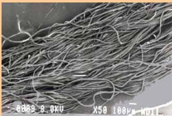
Yarn No.2, salt shrinkage 32.2%, resin uptake 9.5%
