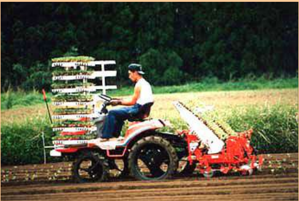
Fig.8. Fully automatic transplanter model SK20 for cell mold seedlings (Kubota, Co., Ltd., used in Takeda, Kumamoto)
