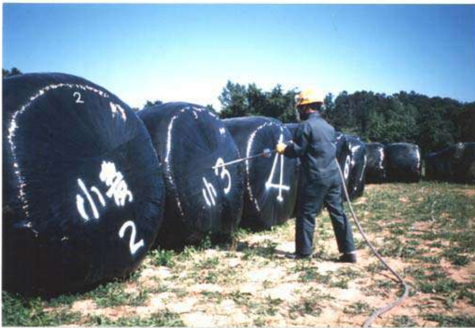
Fig.2. Rapid and safe injection of ammonia
