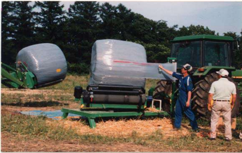
Fig.3 Wrapping of cereal straw with plastic stretch film
