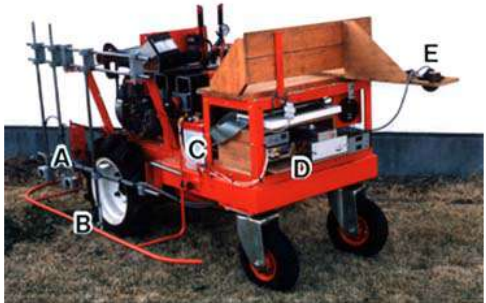
Fig. 8. Experimental vehicle equipped with steering control system
