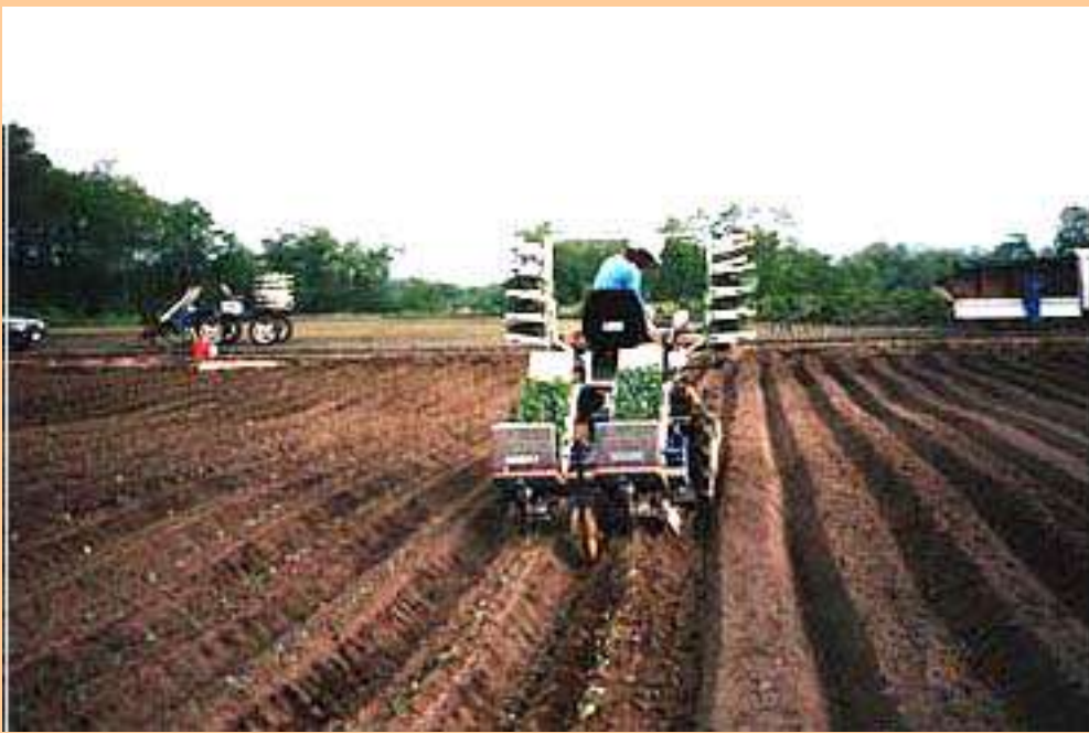
Fig.9. Fully automatic transplanter model PVR200 for pulp mold cell pot seedlings (Iseki Noki, Co., Ltd., used in JA Kazuno, Akita)
