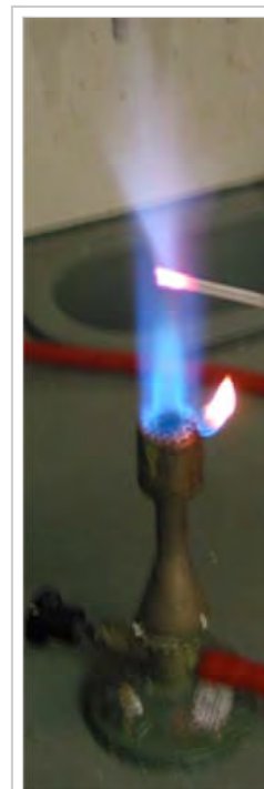
Flame test: lead colors flame pale blue
