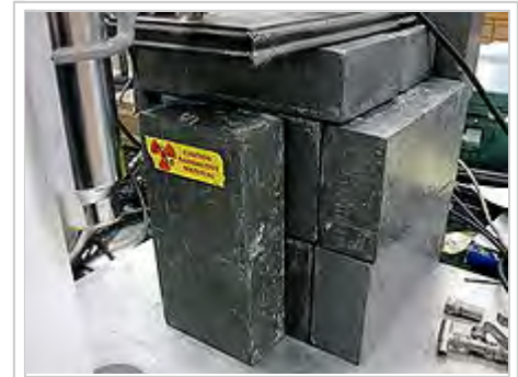
Lead bricks are commonly used as radiation shielding.
