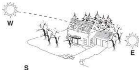
Figure 3 Orient the house to take advantage of winter solar gain and summer shading.
