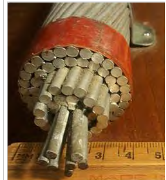
A typical ACSR. The conductor consists of seven strands of steel surrounded by four layers of aluminium.
