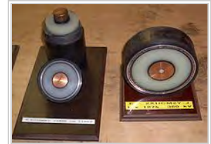
Segments of high-voltage cables
