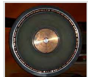
A cross-section through a 400 kV cable, showing the stranded segmented copper conductor in the center, semiconducting and insulating layers, copper shield conductors, aluminum sheath and plastic outer jacket
