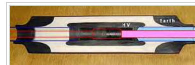
Photograph of a section of a high-voltage joint, bi-manchet , with a high-voltage cable mounted at the right hand side of the device.
