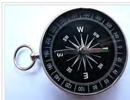
A simple dry magnetic pocket compass
