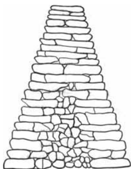
FIG. 87.—Cross-section of a stone fence.
