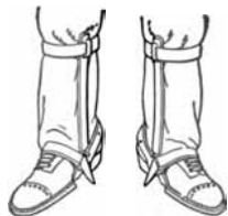
FIG. 34.—Method of attaching climbers or "hooks" to the legs and feet.
