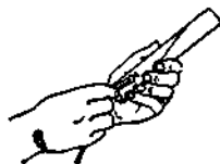
FIG. 60.—Inserting cap in cartridge.
