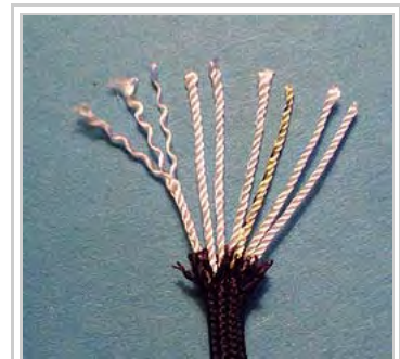
MIL-SPEC MIL-C-5040 Type III Paracord has 7 to 9 inner yarns made up of 3 strands each.
