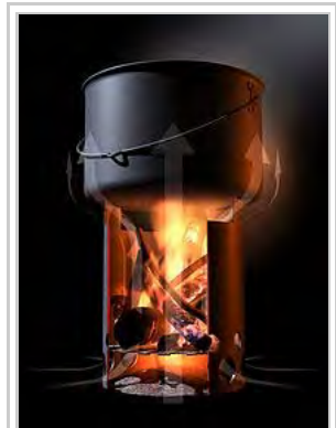
Heat convection in a hobo stove
