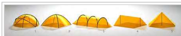
Typical lightweight and trekking tent designs: 1. geodesic tent, 2. dome tent, 3. tunnel tent, 4. ridge tent, 5. pyramid tent
