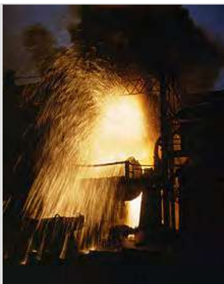
Spray of sparks from a Bessemer converter as air is blown through the molten metal
