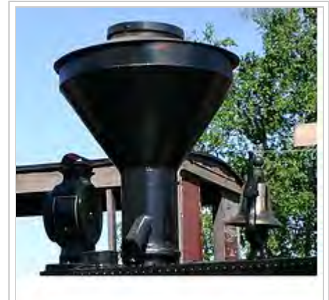
A spark-arresting chimney on a locomotive
