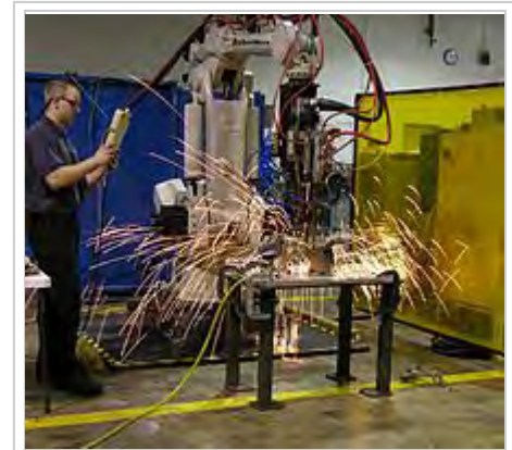
Sparks from spot welding robot
