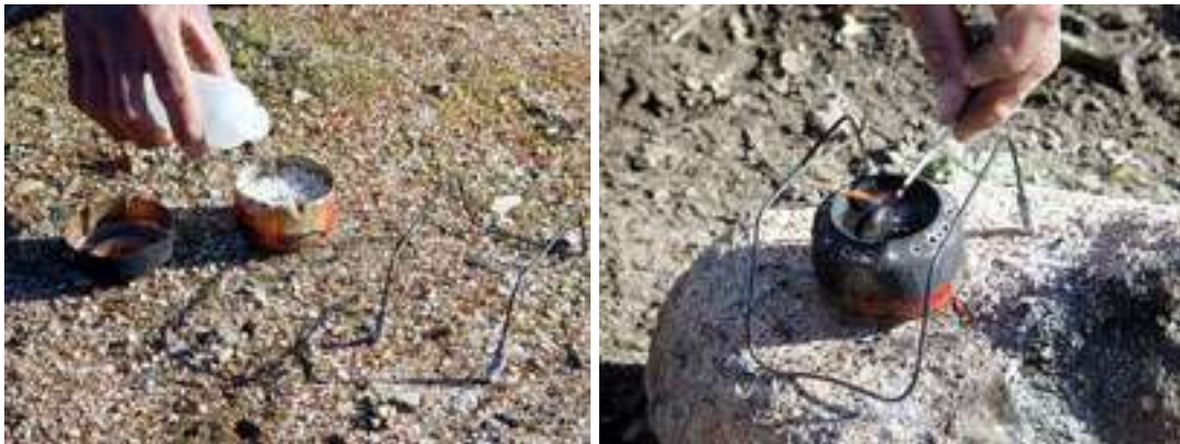
Soda can cooking stove. Clothes hanger wire was used for the pot stand.
