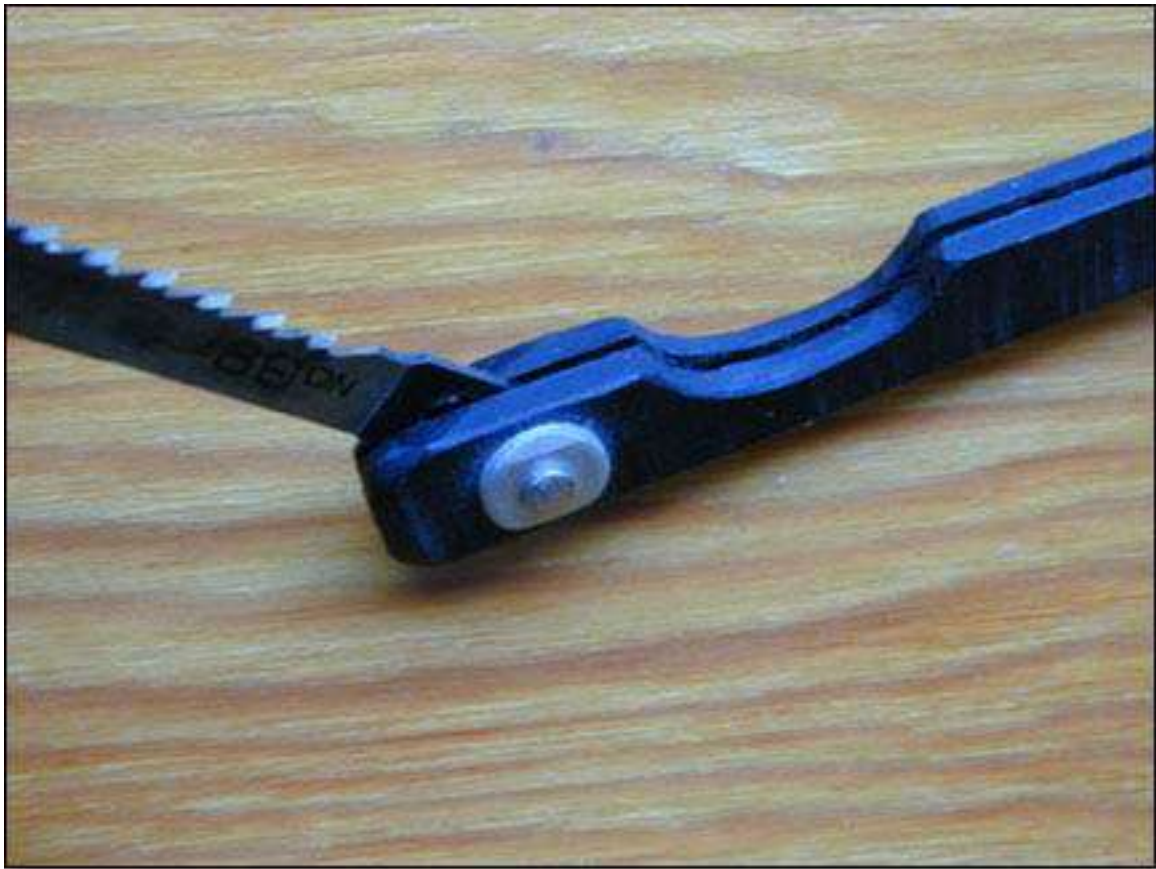
Close-up of riveted area.
