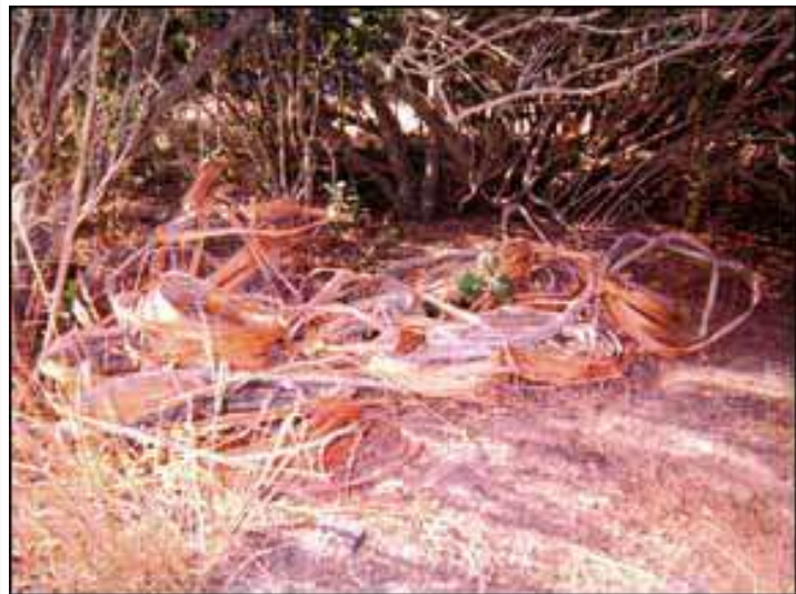
Dried willow bark awaiting final preparation for use in lashing the house frame.
