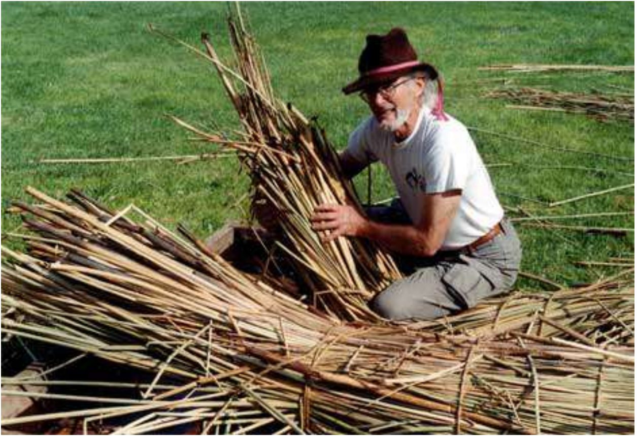
Dick is forming the upward curve on the prow of the tule boat.
