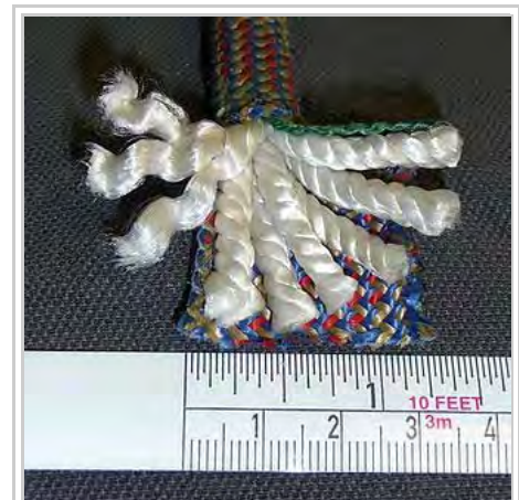
Dynamic Kernmantle rock climbing rope with its braided sheath cut to expose the twisted core yarns and core yarn plies.
