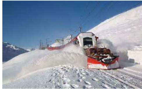
Swiss low-profile, train-mounted snowplow.
