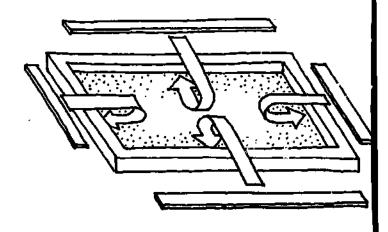
You are likely to find that after using the screen several times it becomes torn or clogs in places with dried ink or other wastes. When this happens you will have to take off the fabric and stretch new material onto the frame.
