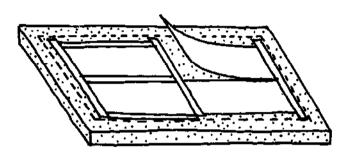
using either lots of gumstrip; or if you have a large area to cover, pieces of unused stencil stuck down with gumstrip. When you have completely masked the screen check that there are no holes where the ink can sneak through, by holding the screen up to the light. Cover any remaining holes with patches of gumstrip.
