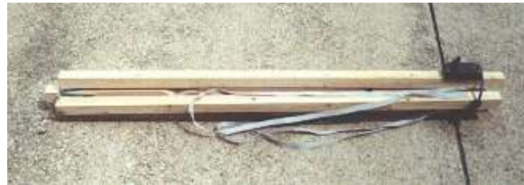
The umbrealla loop folded for transport.
