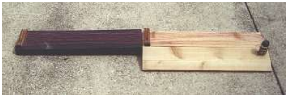
Folding loop antenna - folded.
