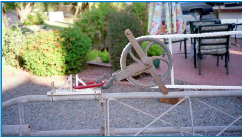
The top of the tower is fitted with this larger pulley.
