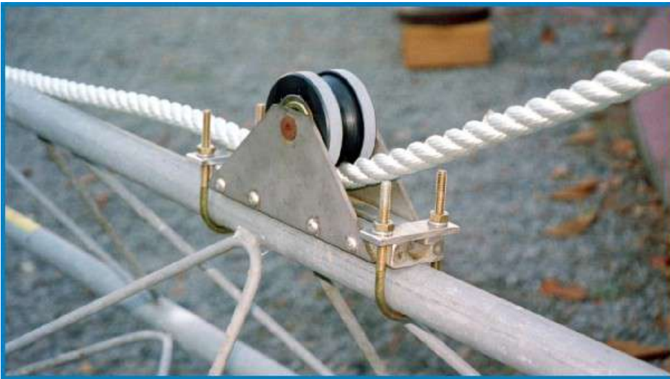
I made this pulley to support the mid section while raising the assembly.
