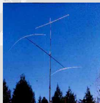
ROTATING FULL SIZE 80 METER 2 ELEMENT QUAD FREESTANDING AT 125 FEET 40 FEET FRONT TO BACK SPACING
