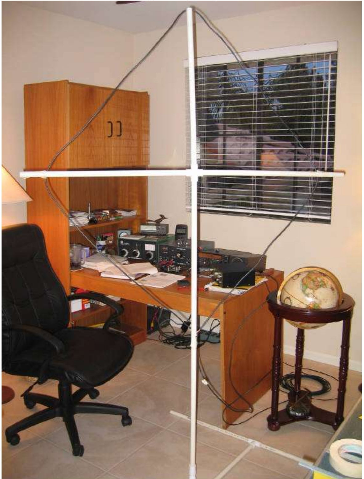
Prototype 40m Loop - works great!
