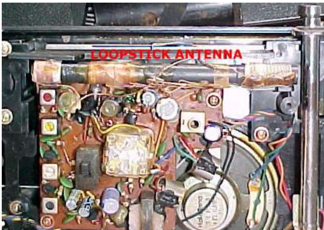
Figure 10. - AM and shortwave loopstick antenna
