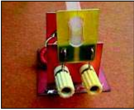
Figure 6 —View of an assembled center insulator fashioned from a 3×3-inch piece of PC board from which all the foil has been removed.
