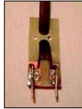
Figure 4—The pad side of the home-made feed-line-to-tuner connector.
