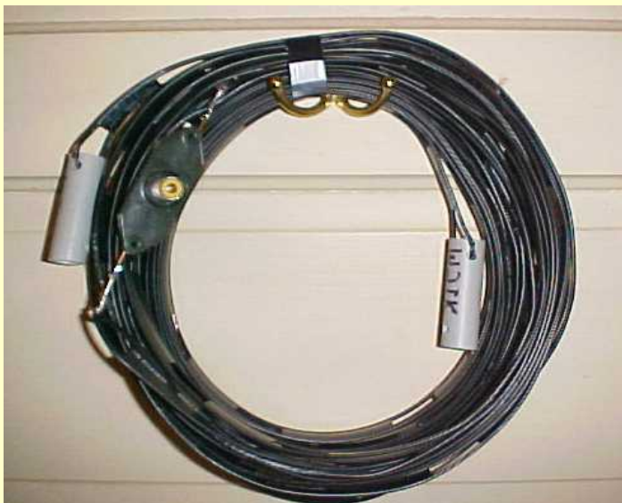
LADDER LINE ANTENNA COILED UP FOR STORING IN A BACK PACK SO IT CAN BE USED WHILE HIKING OR CAMPING
