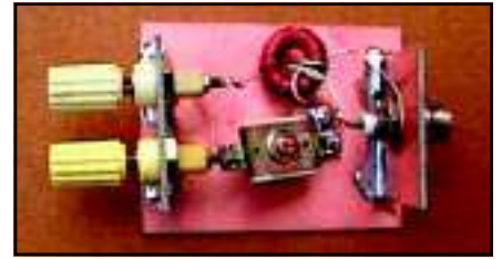
Figure 8 —This Squirt tuner prototype uses a 2×3-inch piece of PC board for the base plate, two 1½×1½-inch pieces for end plates and a ½-inch square piece as a tie point for the toroid and tuning capacitor.
