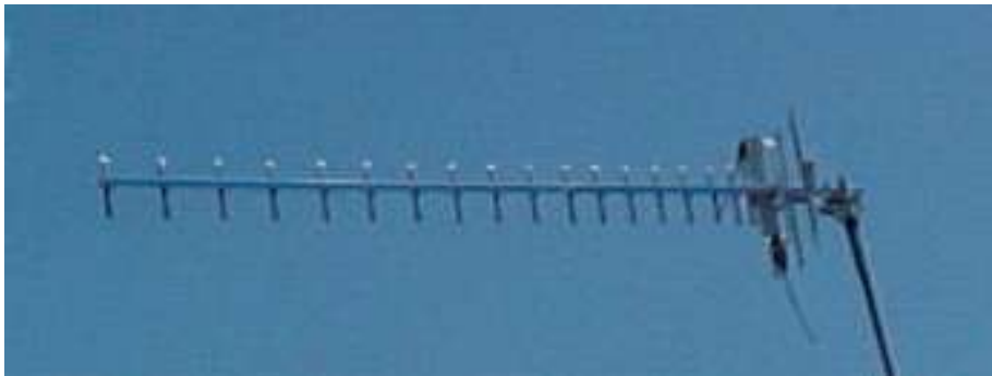
Figure 7. - a vertically polarised UHF Yagi antenna
