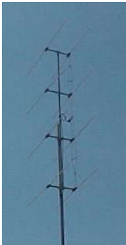
Figure 8. - four stacked half wave dipoles collinear antenna
