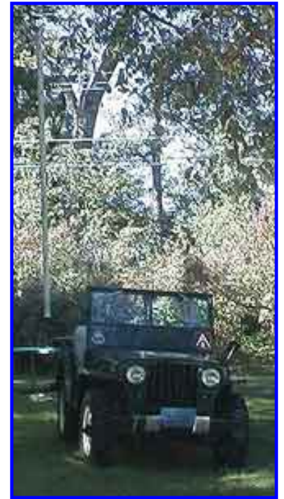
The 10-foot tall, two-inch diameter IFA antenna on N9ZRT's jeep. [N9ZRT Photo]
