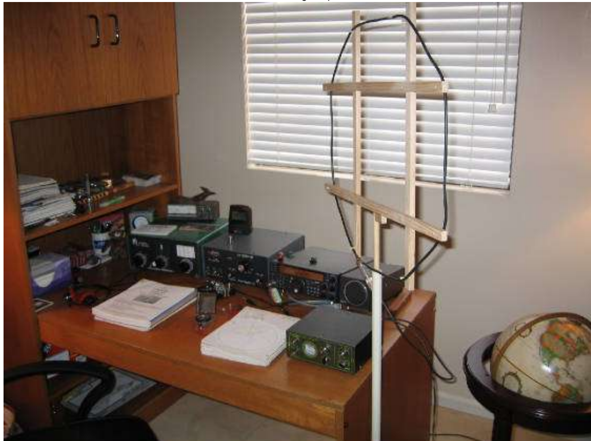
20m HF Receiving Loop Antenna
