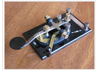
A typical "straight key". This U.S. model, known as the J-38, was manufactured in huge quantities during World War II, and remains in widespread use today. In a straight key, the signal is "on" when the knob is pressed, and "off" when it is released. Length and timing of the dots and dashes are entirely controlled by the telegraphist.
