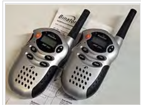
Walkie talkies which operate on the 446 MHz PMR(Professional Mobile Radio) band. The 67 cm wavelength permits them to use very short "Rubber Ducky" antennas.
