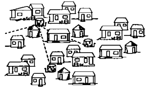
Equal priority multiple tank delivery system
