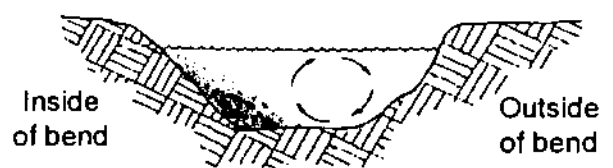
Section through river on a bend
