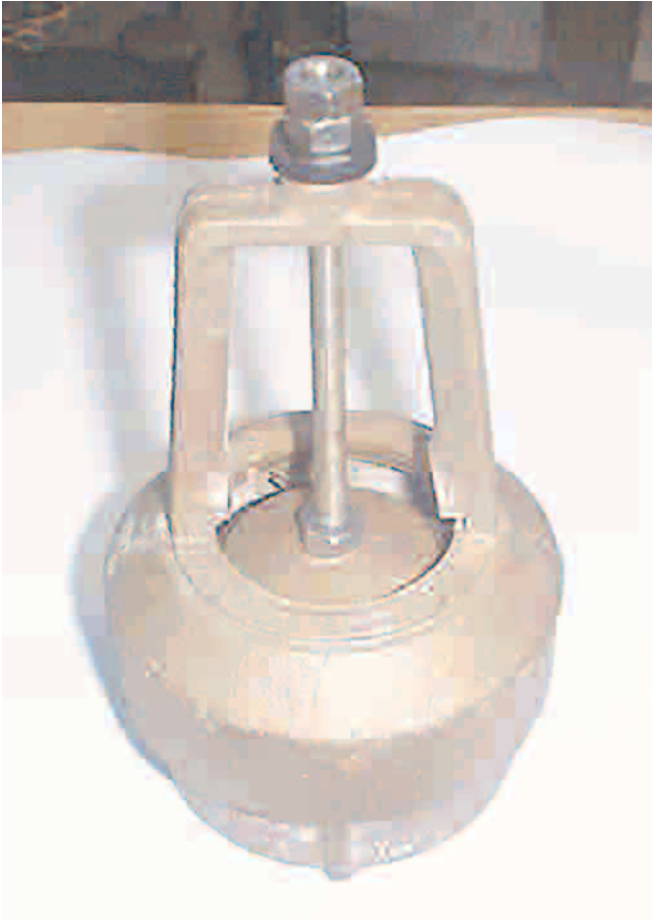
The modified foot valve ready to assemble onto the ram.
