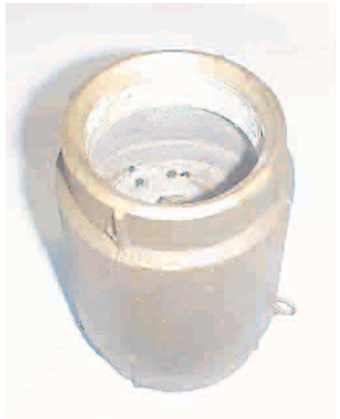
The check valve with the wire poking out of the air sniffer hole.
