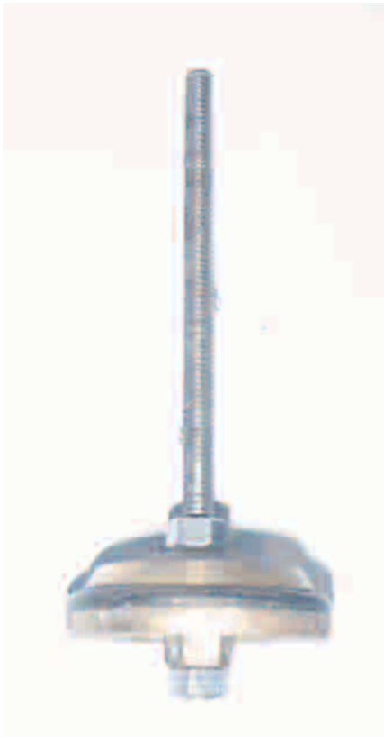
The valve disc is reassembled with a 6 inch long piece of 0.25 inch stainless steel threaded rod, and locked in place with nuts top and bottom.
