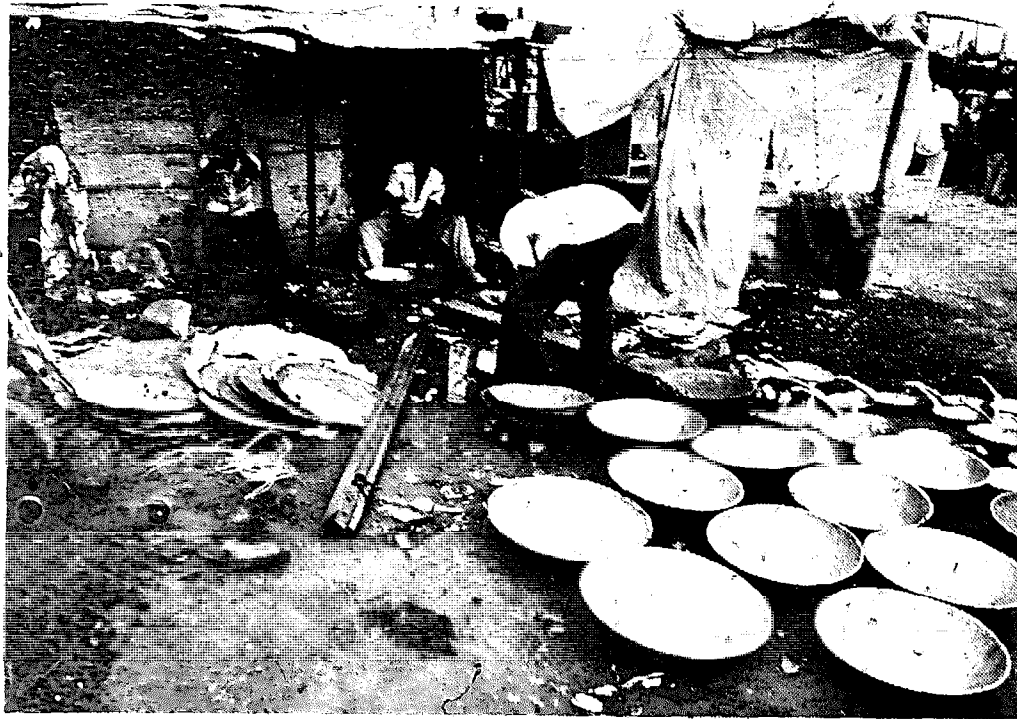
Fig. 19 Manufacture of cooking bowls from oil-drum ends, Kenya.
