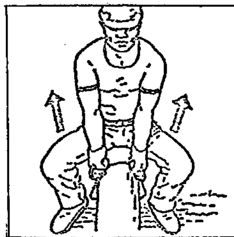
(d) Use two hooks and leg muscles for lifting.
