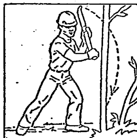
(f) The left hand should be in the upper position when cutting from the left side and vice versa when cutting from the right
