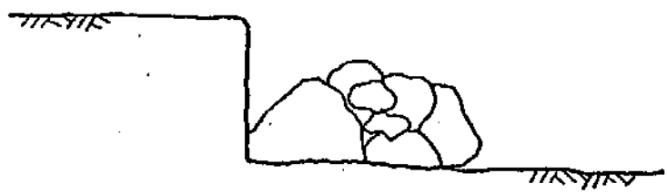
View B-B: Excavated section ready for loading
