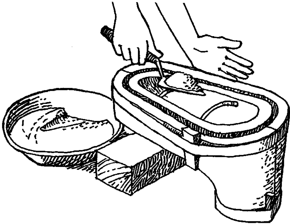
Figure 90 Casting the pan
