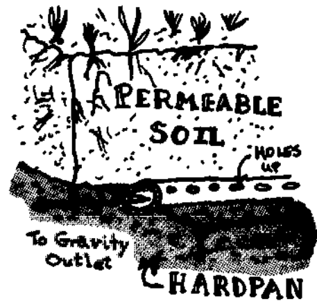
The holes are up to keep soil out of pipe. If you put gravel under curtain drain pipe then the direction of the holes doesn't matter.
