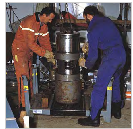
An air gun seismic source (30 litre)
