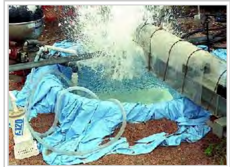
Plasma sound source fired in small swimming pool
