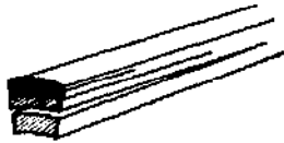
Figure 3.9c Use a knife to split the harder outer strip from the soft, pithy inner strip which is usually discarded.
