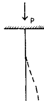
4 Fixed in position and in direction.
