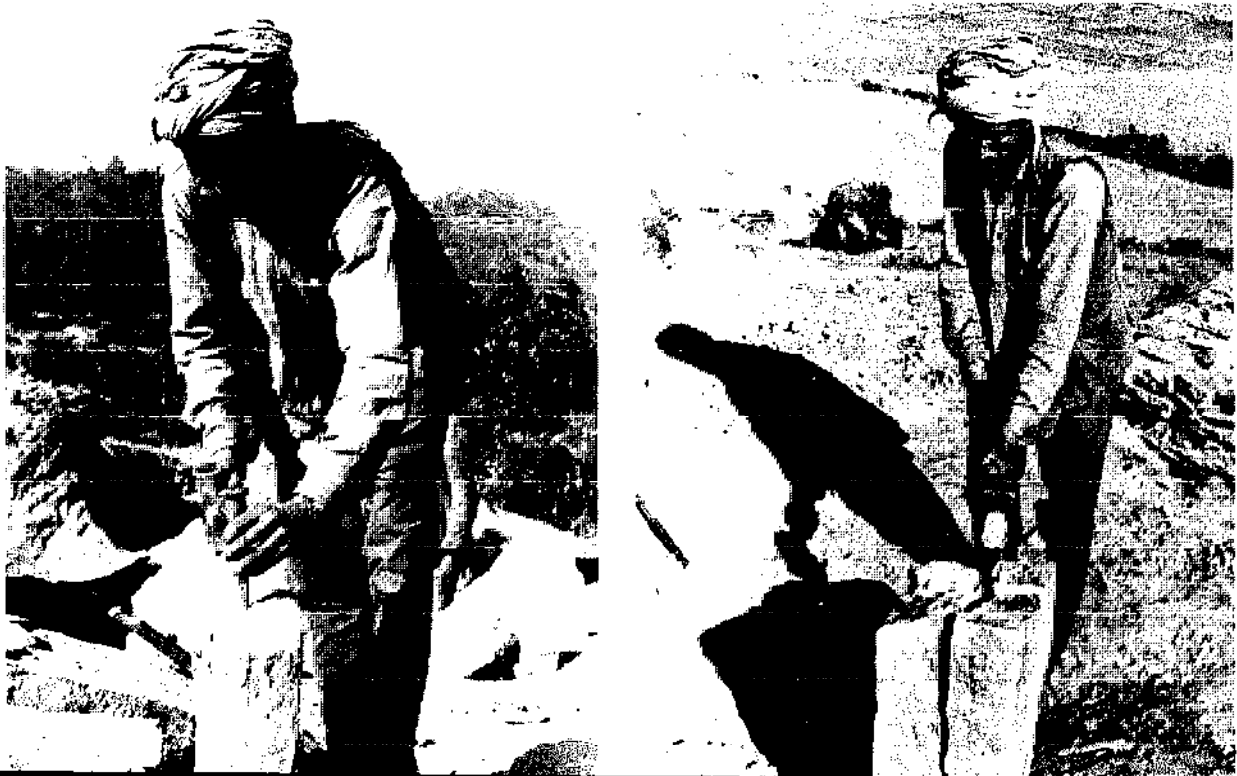
Above: Wedges are inserted into sandstone then split with sledge-hammers in Nepal. Below: Splitting sandstone, first with a hammer and chisel (left) then with a sledge-hammer peen.
