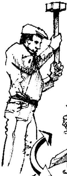
Making holes by hand with a plug drill
