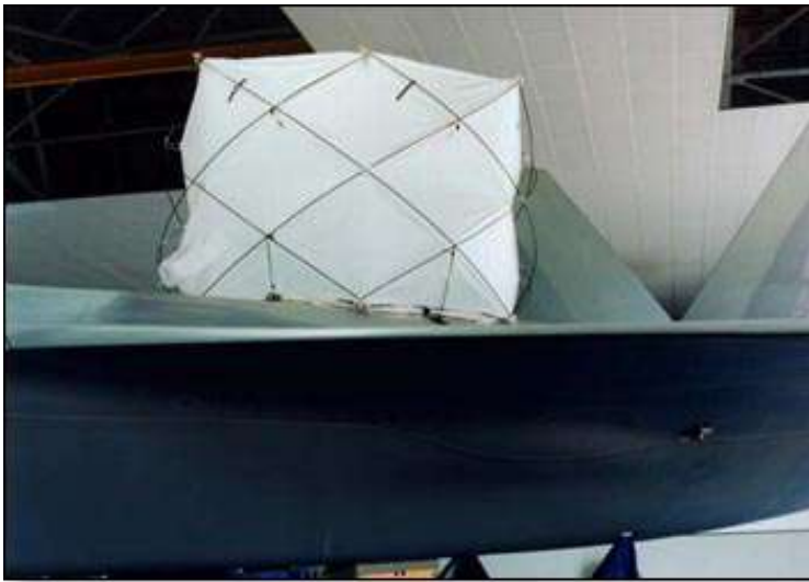
Special Cylindrical Tent for working on panels of the F22.
