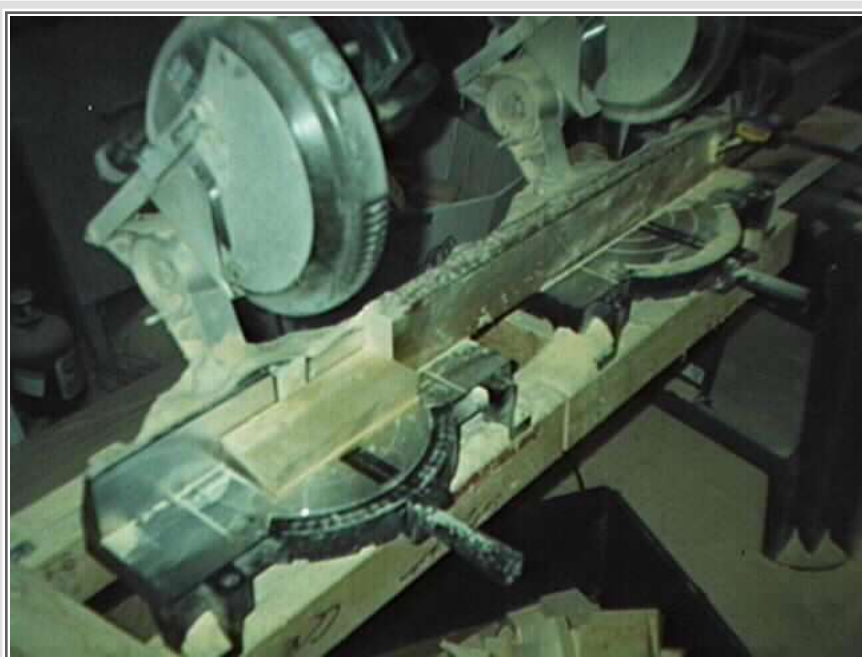
Cut predrilled wedge board in 4 inch increments
