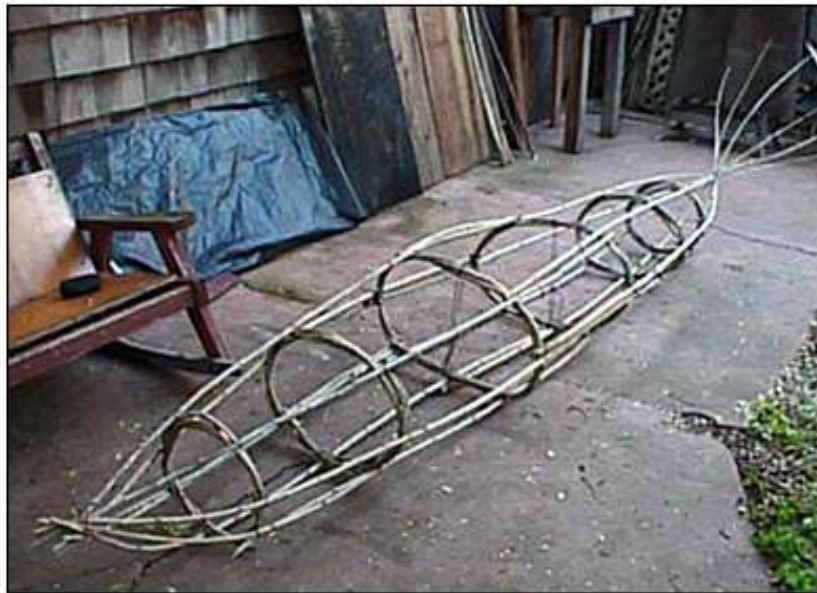
Completed frame side view.
