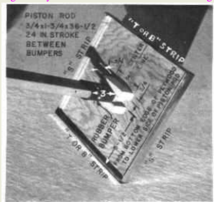
Fig. 14. Plywood Piston with Sheetmetal Sealing Strips Attached.
