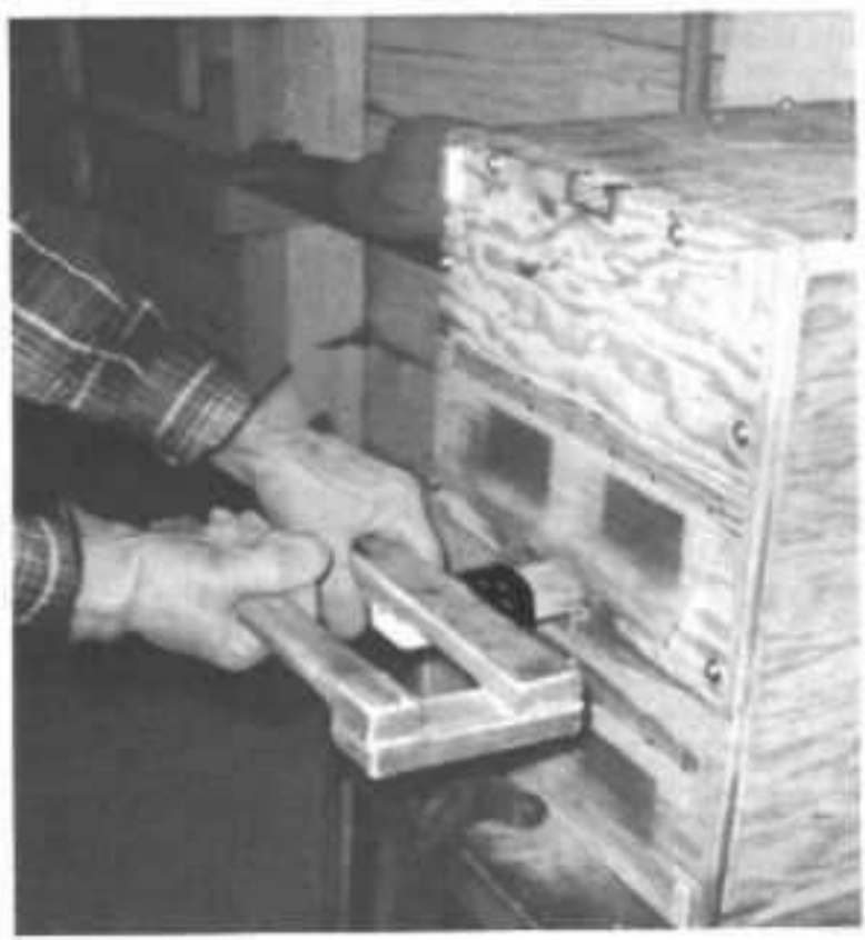
Fig. 15. Piston Rod Handle Made of 3/4 x 1-3/4-in. Boards.
