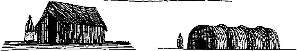
FIG. 2.3. Dwellings made of one material (reeds). Left: Uru dwelling, Lake Titicaca, Peru. Right: Marsh Arab dwelling, Iraq-Iran border.
