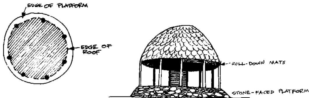
FIG. 3.2. Samoa dwelling, diagrammatic plan and perspective.
