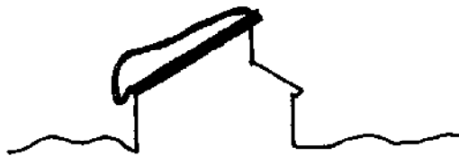
LOW-SLOPE ROOFS HOLD SNOW AND DIRT
